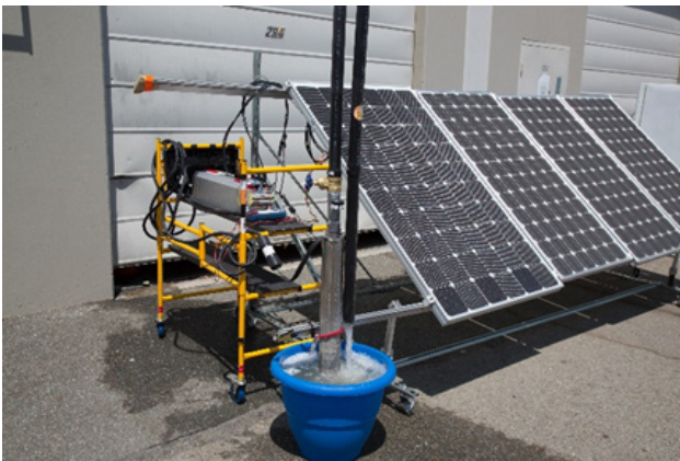
Demonstration unit with PVflex equipped solar PV-modules and brushless DC pump with external pump controller
